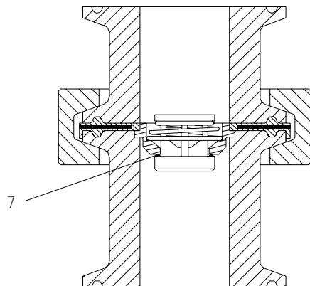
Illustration showing typical design of 3/4"-4" standard units (with exception of 1" HCV04HC). Cartridge valve with soft seat seal fitted shown.
