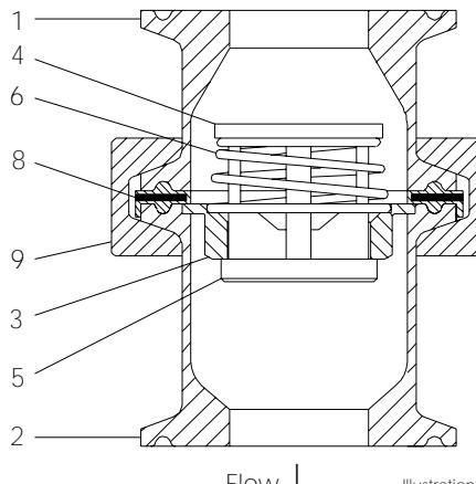
Illustration showing typical design of 1/2" and 1" HCV04HC units with metal-metal seating.
