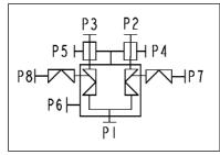
DV2WS with Condensate Drain Valves
