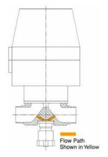
Bypass Flow Path Section
