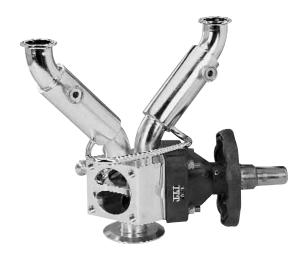
The Sterile Tank Vent Filter Shunt Valve is a steam traced 2-Way divert valve designed to provide the flexibility of changing from one vent filter cartridge to another on WFI storage tanks without interrupting operations.
