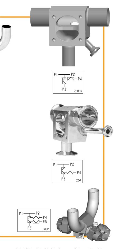
Note: All Zero Static block bodies are available as "T" or "U" bend configurations.
