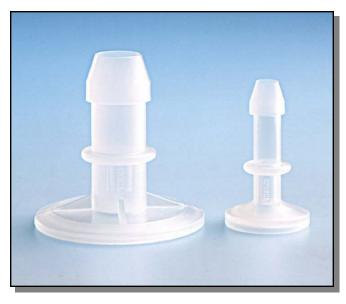
True bore design allows for full flow and no restriction of product transfer. Where flow needs to be calculated, there are no corrections that need to be made. The true bore design through the entire *Bio Barb*® *Adapter* does not promote a venturi in the cavity at the Tri-Clamp® where other adapters may. Eliminating turbulence caused by the adapter reduces possible damage to the medium being transferred.
