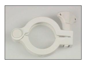
The Heleon group has a complete programme of clamps for the Tri-Clamp connections. These plastic clamps are made of reinforced Polyamide (Nylon). This clamp is specially suitable for clamp applications which require a low force. They match very well with the plastic and Silicone end fittings program of Heleon. Because of its light weight is very practical in small laboratory processes.
