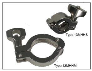
The Heleon group has a complete programme of clamps for the Tri-Clamp connections. These heavy two part clamps are made of solid Stainless Steel with a smooth surface finish. Through the sound double pin construction, the clamp is suitable for every purpose. These clamps match perfectly with many US OD, ISO and DIN Tri-Clamp sizes. The clamp is standard supplied with a solid wing nut and packed properly.
