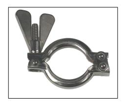
The Heleon group has a complete programme of clamps for the Tri-Clamp connections. These light two part clamps are made of deformed sheet material and hinged with a double pin construction, which makes this clamp easy to use. This light weight clamp is more tolerant on the flange thickness and is intended for lower line pressures.
