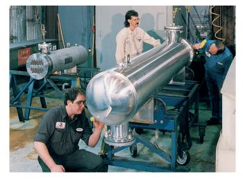
Allegheny Bradford's on-site electropolishing services will deliver the ultra-smooth finish your processing demands, regardless of the design and size of your heat exchanger. Our advanced proprietary techniques are designed to increase corrosion resistance, remove contaminants, maximize passivation and reduce surface friction.
